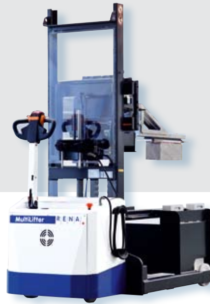
Brick transport system MultiLifter
