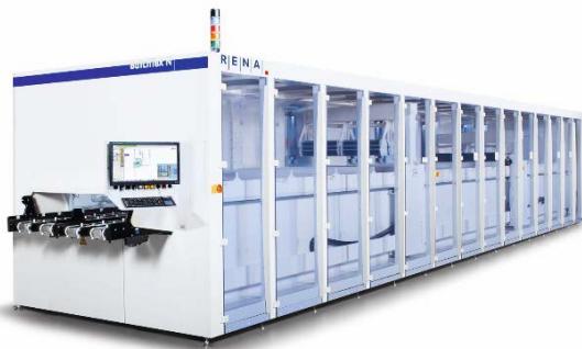
RENA BatchTex N400: Equipment for alkaline texturing of monocrystalline silicon
