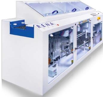
Inline prototype. The tool is based on a similar concept like the inline tools used for mass-production of solar cells.
