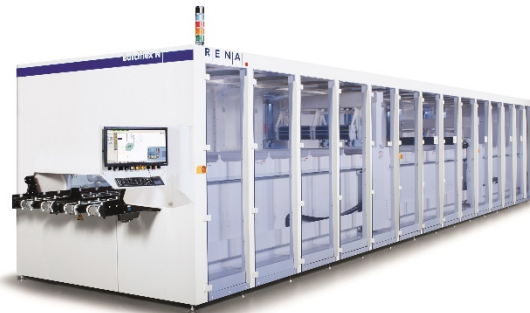
RENA BatchTex N400-8000: Newest release of the industry standard texturing tool with 30% higher throughput → up to 8000 wafer/hour in a single machine.
